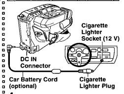
Connect PV-C16 <u>Car Battery Cord</u> (optional) to Camcorder DC IN.
