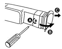
A Remove the screw with a Phillips screwdriver.
